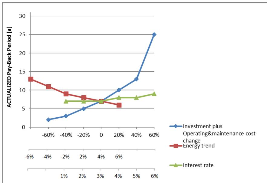
Figure 1b. Sensitivity of Payback to changes in economic parameters for an nZEB package for a Croatian office (Continental climate)
