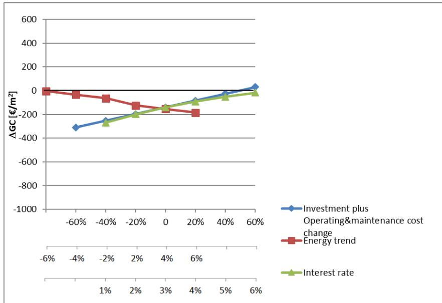
Figure 1a. Sensitivity of Global Cost to changes in economic parameters for an nZEB package for a Croatian office (Continental climate)
